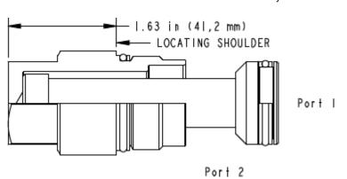
Sun filter elements are available as Surface Type (Last Chance) and Depth Style elements. The flow path is Port 2 to Port 1 and should not be used in reverse, even with a reverse free flow check valve installed. The elements have a high collapse pressure and are intended to be used in line with the system. Filter life will depend on initial system cleanliness and the amount of dirt ingression to the system when operating.
