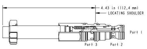
This valve is a 3-way, meter-in, electro-proportional throttle. The flow path, unenergized, has the supply blocked at port 1 and port 2 is drained to tank at port 3. Energizing the coil generates a closing force on the spool, creating a metering orifice in the 1 to 2 direction that is proportional to the coil command current. The valve self-compensates in the 1-to-2 direction and with the addition of an external compensator
