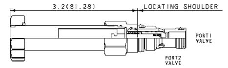
This valve is a pilot-operated, normally closed, electro-proportional throttle with reverse free-flow check. Energizing the coil generates an opening force on the pilot stage which vents the main stage poppet to open proportionally, allowing flow from port 2 to 1. In the open condition, flow from 1 to 2 will cause the valve to autoclose and only pilot flow will pass from 1 to 2.
