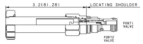
This valve is a pilot-operated, normally closed, electro-proportional throttle with reverse free-flow check. Energizing the coil generates an opening force on the pilot stage which vents the main stage poppet to open proportionally, allowing flow from port 2 to 1. In the open condition, flow from 1 to 2 will cause the valve to autoclose and only pilot flow will pass from 1 to 2.
