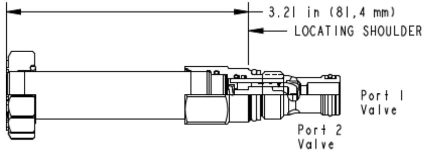
This valve is a pilot-operated, normally open, electro-proportional throttle with reverse free-flow check. Energizing the coil generates a closing force on the pilot stage which pushes the main stage poppet against the seat, proportionally blocking flow from port 2 to 1. In the open condition, flow from 1 to 2 will cause the valve to auto-close and only pilot flow will pass from 1 to 2.
