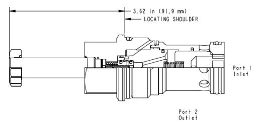
This valve is a pilot-operated, normally closed, electro-proportional throttle with reverse free-flow check. Energizing the coil generates an opening force on the pilot stage which vents the main stage poppet to open proportionally. Metered flow is from port 1 to port 2 with reverse free flow from port 2 to port 1.
