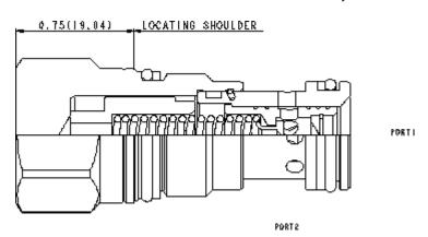
Flow fuse cartridges are used to maintain the position of a hydraulic actuator in the event of a hose or line break. The valve allows flow to and from the actuator but closes instantly if flow from the actuator exceeds the setting of the valve. NOTE: Because the valve responds so rapidly, it is sensitive to any transient flow above the valve setting.
