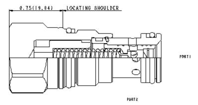
Flow fuse cartridges are used to maintain the position of a hydraulic actuator in the event of a hose or line break. The valve allows flow to and from the actuator but closes instantly if flow from the actuator exceeds the setting of the valve. NOTE: Because the valve responds so rapidly, it is sensitive to any transient flow above the valve setting.
