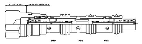
High accuracy, closed-center flow divider/combiners are sliding-spool, pressure-compensated devices used to split flow in one direction and combine flow in the opposite direction. These valves may be used to accurately control two or more cylinders or hydraulic motors where bidirectional operation is required.
