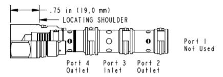
Flow dividers are sliding-spool, pressure-compensated devices used to split oil flow to two different branches of a circuit in a designated ratio. These valves are suitable for
