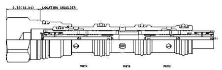
Closed-center flow divider/combiners are sliding-spool, pressure-compensated devices used to split flow in one direction and combine flow in the opposite direction. These valves may be used to accurately control two or more cylinders or hydraulic motors where bidirectional operation is required.
