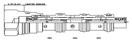
High-capacity, closed-center flow divider/combiners are sliding-spool, pressure-compensated devices used to split flow in one direction and combine flow in the opposite direction. These valves have approximate 15% greater capacity than standard closed-center divider/combiners and are designed for use in tractive drive systems. Note: Accuracy on these cartridges is not equivalent to the accuracy of standard closed-center divider/combiners.
