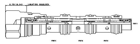
Synchronizing flow divider/combiners are sliding-spool, pressure-compensated devices used to split flow in one direction and combine flow in the opposite direction. With a sychronizing feature, these valves can be used to allow two hydraulic cylinders to fully stroke and synchronize at the end of the stroke. When the first cylinder has reached the end of its stroke, a pressure-compensated, reduced flow is metered to or from the second cylinder until it also reaches the end of its stroke.
