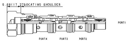
Closed-center flow divider/combiners are sliding-spool, pressure-compensated devices used to split flow in one direction and combine flow in the opposite direction. These valves may be used to accurately control two or more cylinders or hydraulic motors where bidirectional operation is required.
