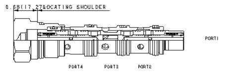
High accuracy, closed-center flow divider/combiners are sliding-spool, pressure-compensated devices used to split flow in one direction and combine flow in the opposite direction. These valves may be used to accurately control two or more cylinders or hydraulic motors where bidirectional operation is required.
