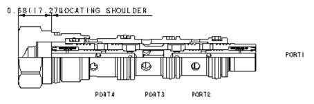
High-capacity, closed-center flow divider/combiners are sliding-spool, pressure-compensated devices used to split flow in one direction and combine flow in the opposite direction. These valves have approximate 15% greater capacity than standard closed-center divider/combiners and are designed for use in tractive drive systems. Note: Accuracy on these cartridges is not equivalent to the accuracy of standard closed-center divider/combiners.
