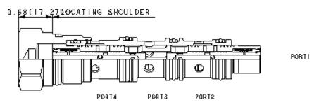
Synchronizing flow divider/combiners are sliding-spool, pressure-compensated devices used to split flow in one direction and combine flow in the opposite direction. With a sychronizing feature, these valves can be used to allow two hydraulic cylinders to fully stroke and synchronize at the end of the stroke. When the first cylinder has reached the end of its stroke, a pressure-compensated, reduced flow is metered to or from the second cylinder until it also reaches the end of its stroke.
