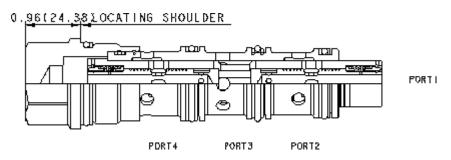
Closed-center flow divider/combiners are sliding-spool, pressure-compensated devices used to split flow in one
