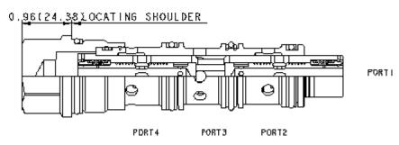
Closed-center flow divider/combiners are sliding-spool, pressure-compensated devices used to split flow in one
