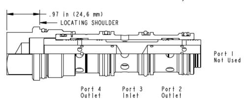
Flow dividers are sliding-spool, pressure-compensated devices used to split oil flow to two different branches of a circuit in a designated ratio. These valves are suitable for applications that use the following: unidirectional hydraulic motors, hydraulic cylinders where flow division in one direction only is required, and multiple circuits that are serviced from one pump supply.
