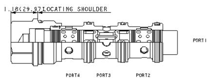
Closed-center flow divider/combiners are sliding-spool, pressure-compensated devices used to split flow in one direction and combine flow in the opposite direction. These valves may be used to accurately control two or more cylinders or hydraulic motors where bidirectional operation is required.
