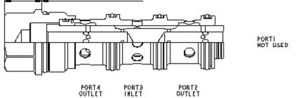
Flow dividers are sliding-spool, pressure-compensated devices used to split oil flow to two different branches of a circuit in a designated ratio. These valves are suitable for applications that use the following: unidirectional hydraulic motors, hydraulic cylinders where flow division in one direction only is required, and multiple circuits that are serviced from one pump supply.
