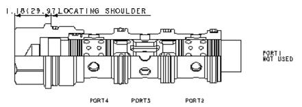
Synchronizing flow divider/combiners are sliding-spool, pressure-compensated devices used to split flow in one direction and combine flow in the opposite direction. With a sychronizing feature, these valves can be used to allow two hydraulic cylinders to fully stroke and synchronize at the end of the stroke. When the first cylinder has reached the end of its stroke, a pressure-compensated, reduced flow is metered to or from the second cylinder until it also reaches the end of its stroke.
