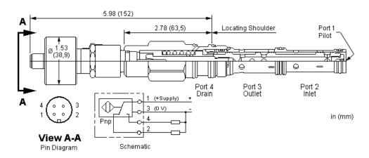
This valve is a 2-way, 2-position proportional throttle. Ports 2 and 3 are normally closed. Pilot pressure at port 1 creates a metering orifice between port 2 and 3 that is proportional to the pressure at 1. The metering passage is self-compensating. This valve uses a dual-path design. Ports 2 and 3 incorporate a double-port area. This valve incorporates a position switch to provide confirmation that the valve is closed.
