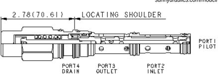
This valve is a 2-way, 2-position proportional throttle. Ports 2 and 3 are normally closed. Pilot pressure at port 1 opposes the spring and creates a variable metering orifice between port 2 and 3 that is proportional to the pressure at 1. The force balance of the flow forces, spring and pilot pressure
