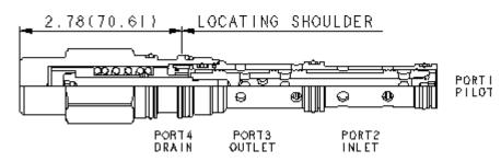
This valve is a 2-way, 2-position proportional throttle. Ports 2 and 3 are normally closed. Pilot pressure at port 1 opposes the spring and creates a variable metering orifice between port 2 and 3 that is proportional to the pressure at 1. The force balance of the flow forces, spring and pilot pressure
