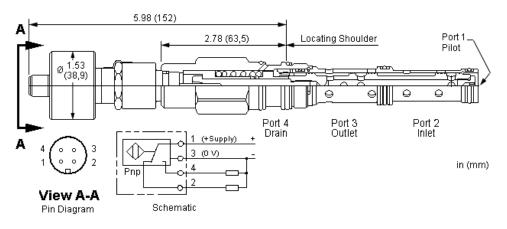
This valve is a 2-way, 2-position proportional throttle. Ports 2 and 3 are normally closed. Pilot pressure at port 1 creates a metering orifice between port 2 and 3 that is proportional to the pressure at 1. The metering passage is self-compensating. This valve uses a dual-path design. Ports 2 and 3 incorporate a double-port area. This valve incorporates a position switch to provide confirmation that the valve is closed.
