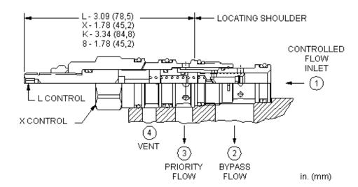
Ventable, bypass/restrictive, fixed-orifice, priority flow controls take an input flow at port 1 and use it to satisfy the priority flow at port 3. If the input flow exceeds the priority flow requirement, the excess is bypassed out port 2. The bypass flow may be used in a secondary circuit. A vent port (port 4) allows these valves to be controlled remotely.
