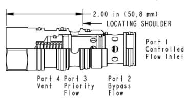
Ventable, bypass/restrictive, fixed-orifice, priority flow controls take an input flow at port 1 and use it to satisfy the priority flow at port 3. If the input flow exceeds the priority flow requirement, the excess is bypassed out port 2. The bypass flow may be used in a secondary circuit. A vent port (port 4) allows these valves to be controlled remotely.
