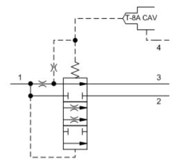
Locating Shoulder 2.0(50.8) T-8A Cavity Accepts Sun's CONTROLLED 2 port Pilot T FLOW Control Cartridges INLET Pilot Control Cartridge (1)Sold Separately 4 VENT (2)3 PRIORITY BYPASS FLOW FLOW in. (mm)
