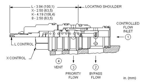
Ventable, bypass/restrictive, fixed-orifice, priority flow controls take an input flow at port 1 and use it to satisfy the priority flow at port 3. If the input flow exceeds the priority flow requirement, the excess is bypassed out port 2. The bypass flow may be used in a secondary circuit. A vent port (port 4) allows these valves to be controlled remotely.
