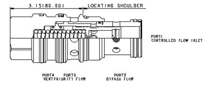
Ventable, bypass/restrictive, fixed-orifice, priority flow controls take an input flow at port 1 and use it to satisfy the priority flow at port 3. If the input flow exceeds the priority flow requirement, the excess is bypassed out port 2. The bypass flow may be used in a secondary circuit. A vent port (port 4) allows these valves to be controlled remotely.
