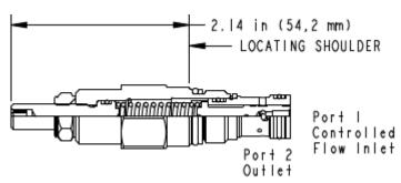
Fixed-orifice, pressure-compensated flow controls provide precise flow regulation for meter-in or meter-out applications where there may be wide pressure fluctuations. The flow setting is specified by the user and is set at the factory.
