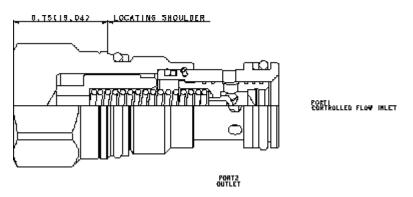
Fixed-orifice, pressure-compensated flow controls provide precise flow regulation for meter-in or meter-out applications
