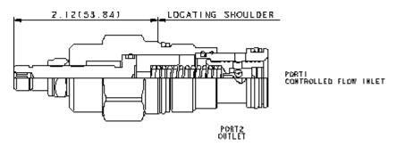
Fixed-orifice, pressure-compensated flow controls provide precise flow regulation for meter-in or meter-out applications where there may be wide pressure fluctuations. The flow setting is specified by the user and is set at the factory.
