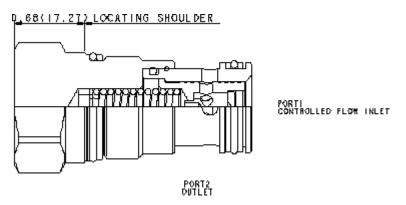
Fixed-orifice, pressure-compensated flow controls provide precise flow regulation for meter-in or meter-out applications where there may be wide pressure fluctuations. The flow setting is specified by the user and is set at the factory.
