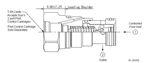
This valve is a fixed-orifice, pressure-compensated flow control valve with an integral pilot control cavity. The pilot control cavity will accept any T-8A pilot control cartridge. This type of valve provides precise flow regulation for meter-in or meter-out applications where there may be wide pressure fluctuations. The flow setting is specified by the user and is set at the factory.
