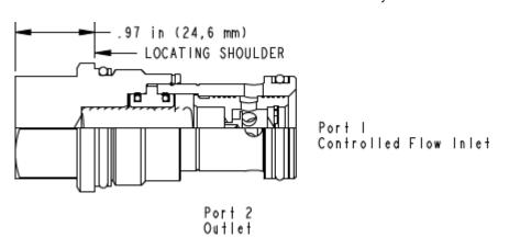
Fixed-orifice, pressure-compensated flow controls provide precise flow regulation for meter-in or meter-out applications where there may be wide pressure fluctuations. The flow setting is specified by the user and is set at the factory.
