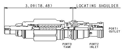
The relief-before-check cartridge is a CavitySaver™ (multi-function) valve incorporating a direct-acting relief tee'd in before a check function. When the pressure at the inlet (port 2) reaches the relief valve setting, the valve starts to open to tank (port 3), throttling flow to limit the pressure rise. The check valve flow is from the inlet (port 2) to the system port (port1). These valves are smooth and quiet, essentially zero leak, dirt tolerant, immune to silting and are very fast.
