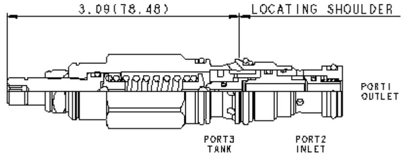
The relief-after-check cartridge is a CavitySaver™ (multi-function) valve incorporating a direct-acting relief tee'd in after a check function. The check valve flow is from the inlet (port 2) to the system port (port1). When the pressure in the system (port 1) reaches the relief valve setting, the valve starts to open to tank (port 3), throttling flow to limit the pressure rise. These valves are smooth and quiet, essentially zero-leak, dirt-tolerant, immune to silting and are very fast.
