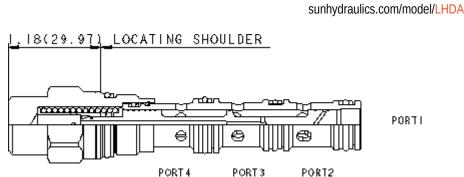
Bypass/restrictive modulating elements, when combined with an external orifice, create a bypass/restrictive flow control. Input flow (port 3) is directed to the priority or control flow at
