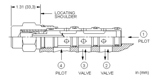
These bi-directional, normally open, modulating elements used with an external orifice, create a bi-directional, pressure compensated flow control.
