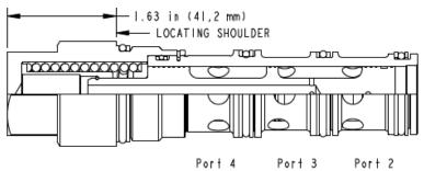
Bypass/restrictive modulating elements, when combined with an external orifice, create a bypass/restrictive flow control. Input flow (port 3) is directed to the priority or control flow at port 2. Once the priority requirements are met, excess flow is bypassed out port 4. The after-orifice signal is connected to port 1. The before-orifice design
