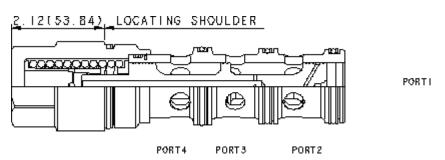
Bypass/restrictive modulating elements, when combined with an external orifice, create a bypass/restrictive flow control. Input flow (port 3) is directed to the priority or control flow at port 2. Once the priority requirements are met, excess flow is
