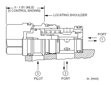
These unbalanced poppet, logic valves are 2-way switching elements that are spring-biased closed. Pressure at either work port 1 or 2 will further bias the valve to the closed position while pressure at port 3 will tend to open it. The force generated at port 3 must be greater than the sum of the forces acting at port 1 and port 2 plus the spring force for the valve to open. NOTE: The pilot area (port 3) is 1.8 times the area at port 1 and 2.25 times the area at port 2.
