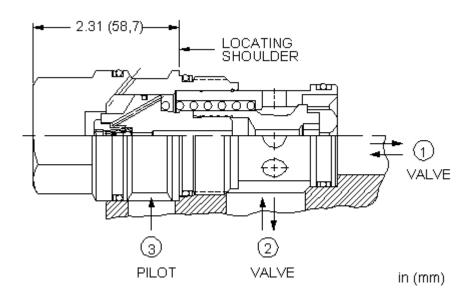
These unbalanced poppet, logic valves are 2-way switching elements that are spring-biased closed. Pressure at either work port 1 or 2 will further bias the valve to the closed position while pressure at port 3 will tend to open it. The force generated at port 3 must be greater than the sum of the forces acting at port 1 and port 2 plus the spring force for the valve to open. NOTE: The pilot area (port 3) is 1.8 times the area at port 1 and 2.25 times the area at port 2.
