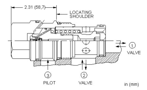
These unbalanced poppet, logic valves are 2-way switching elements that are spring-biased closed. Pressure at either work port 1 or 2 will further bias the valve to the closed position while pressure at port 3 will tend to open it. The force generated at port 3 must be greater than the sum of the forces acting at port 1 and port 2 plus the spring force for the valve to open. NOTE: The pilot area (port 3) is 1.8 times the area at port 1 and 2.25 times the area at port 2.
