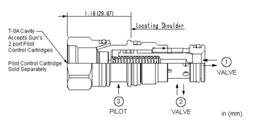
This valve is an unbalanced, vent-to-open, 2-way logic switching element with an integral pilot control cavity. It is spring biased closed and uses port 1 as a pilot source. With
