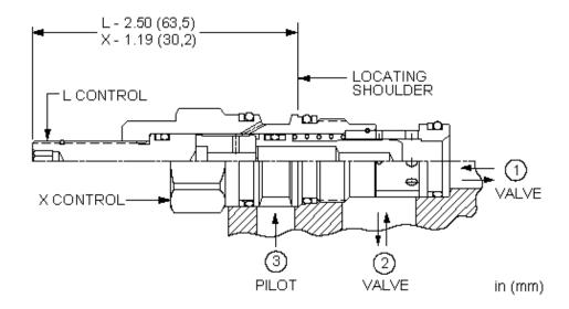
These unbalanced, pilot-to-close logic valves are 2-way switching elements that are spring biased open. Pressure at either work port 1 or 2 will tend to keep the valve open while pressure at port 3 will tend to close it. The force generated at port 3 must be greater than the sum of the forces acting at port 1 and port 2 plus the spring force for the valve to close. NOTE: The pilot area (port 3) is 1.8 times the area at port 1 and 2.25 times the area at port 2.
