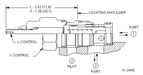
These unbalanced, pilot-to-close logic valves are 2-way switching elements that are spring biased closed. Pressure at either work port 1 or 2 will oppose the spring and tend to open the valve while pressure at port 3 will tend to close it. The force generated at port 3, plus the spring force, must be greater than the sum of the forces acting at port 1 and port 2 for the valve to remain closed. NOTE: The pilot area (port 3) is 1.8 times the area at port 1 and 2.25 times the area at port 2.
